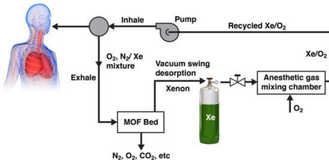
Figure 2 - figure demonstrating a Xenon recycling system.
